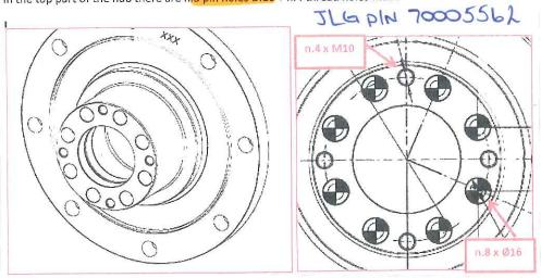
In the rear part of planet carrier there are n.8 pin holes Ø16: ≥
