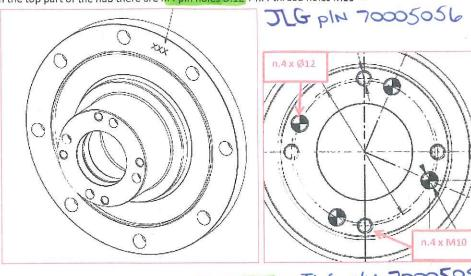
In the rear part of planet carrier there are n.4 pin holes  $\emptyset12$ : = 5LG PN 7000505 $\lambda$
