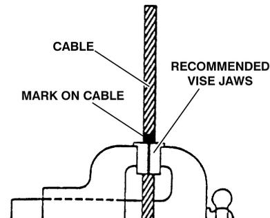
2. Twist the sleeve from the clamp kit onto the rope until it is flat against the vise jaws at the mark made on the wire rope.
