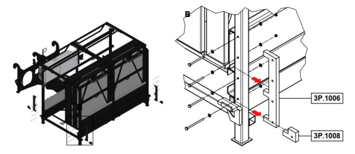
Unscrew bolted connections (BAA7514+BAG4123) from the extension cylinder (3P.1600).
