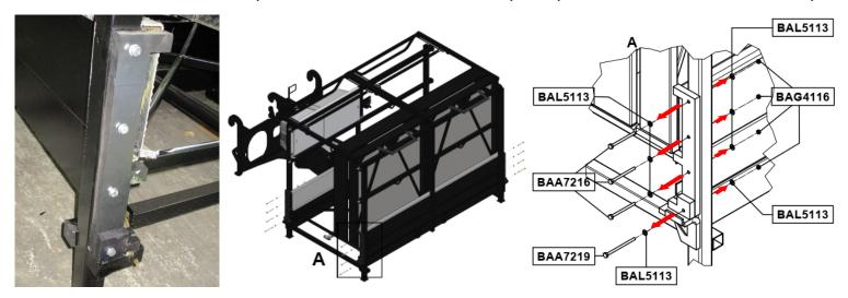
Remove teflon guides (3.P1006) and the reinforcing guides (3P.1008) from fixed frame (3P.1000E).
