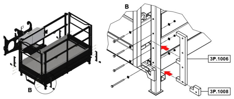
Fix bolted connections (BAA7216+BAL5113+BAG4116) and (BAA7219+BAL5113+BAG4116) to prevent the extensible frames (3P.1202) from coming out. Tightening torque 10 Nm / 7.375 ft/lb
