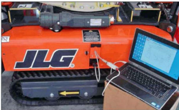
Figure 8-1 RamHino Laptop Connection to the Compact Crawler
