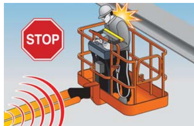
Horn sounds upon operator contact with the bar.
