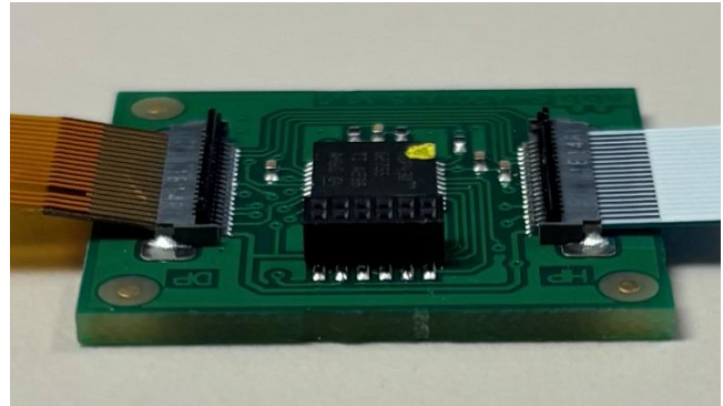
FIGURE 1 07320200 Connector Board with open ribbon cable clamps
